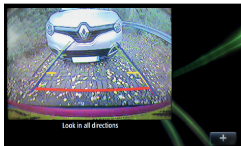
Reverse parking camera system Rear parking sensors with reverse parking camera, which displays the image on the navigation system screen alongside guidance aids.
